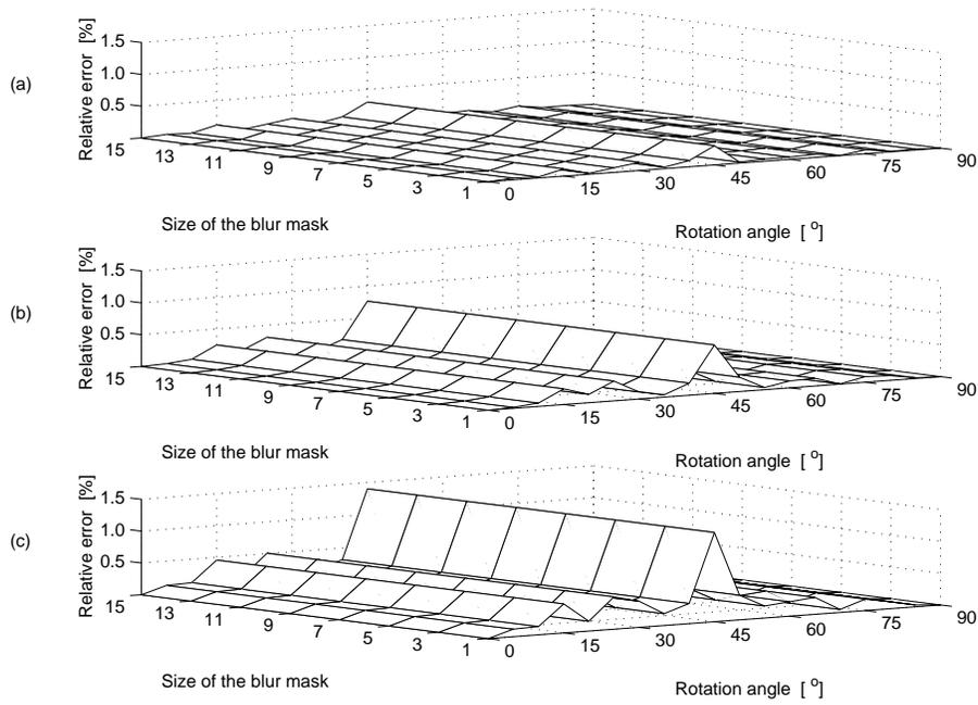
Fig. 2. The relative errors of the invariants for blurred and rotated images. The angle of the image rotation is from  $0^\circ$  to  $90^\circ$ , the size of the blurring filters is from  $1 \times 1$  (no blur) to  $15 \times 15$ . (a)  $\Phi(2, 1)$ , (b)  $\Phi(4, 1)$ , (c)  $\Phi(7, 0)$ .
