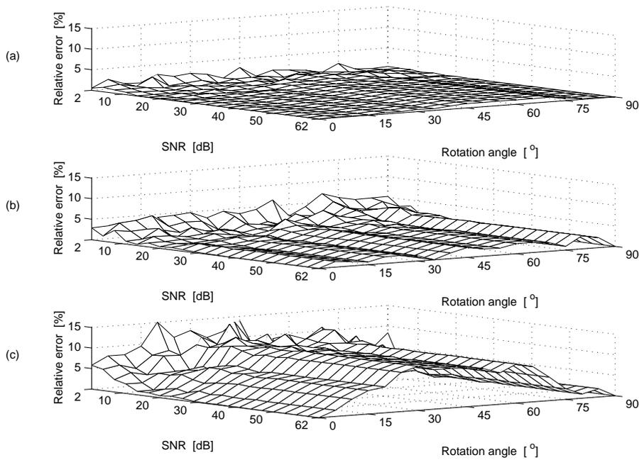
Fig. 3. The relative error of the invariants for blurred and noisy images. The angle of the image rotation is from  $0^\circ$  to  $90^\circ$ , the SNR is from 2 dB to 62 dB. (a)  $\Phi(2, 1)$ , (b)  $\Phi(4, 1)$ , (c)  $\Phi(7, 0)$ .
