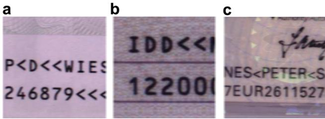
Fig. 1. Images from the DocuCenter: (a) A part of the MRZ correctly captured. (b) The MRZ with cropped last characters. (c) Several letters are made defective by the hologram reflection.
