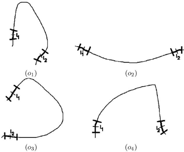
Fig. 10.  $I_1, I_2$  labels in every image the original points of inflection. We computed the penalty function between the image with original inflection points and the images, where the inflection points were chosen from the highlighted interval. The size of the interval is 10% of the length of original border.
