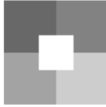
Fig. 1. Partition of tile image into five regions. The texture is analysed in the whole image and separately in these regions.
