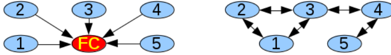
Figure 1: Principles of centralized and decentralized schemes. The centralized one (left) embodies a fusion center (FC) responsible for computation of estimates; in the decentralized concept (right) the computation task lies on the network nodes disseminating the available information, possibly partial. Remind, that the network topology of the decentralized scheme may differ from case to case.
