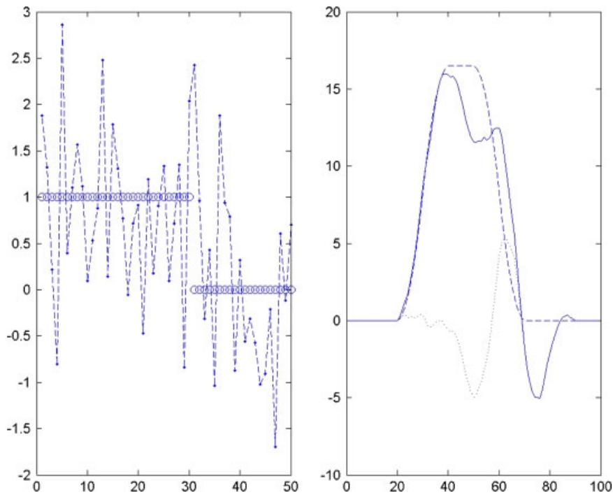
Figure 2. Left: signal (circles) and signal with noise (dots). Right: filtered signal (dashed), noise (dotted), and signal with noise (full).
