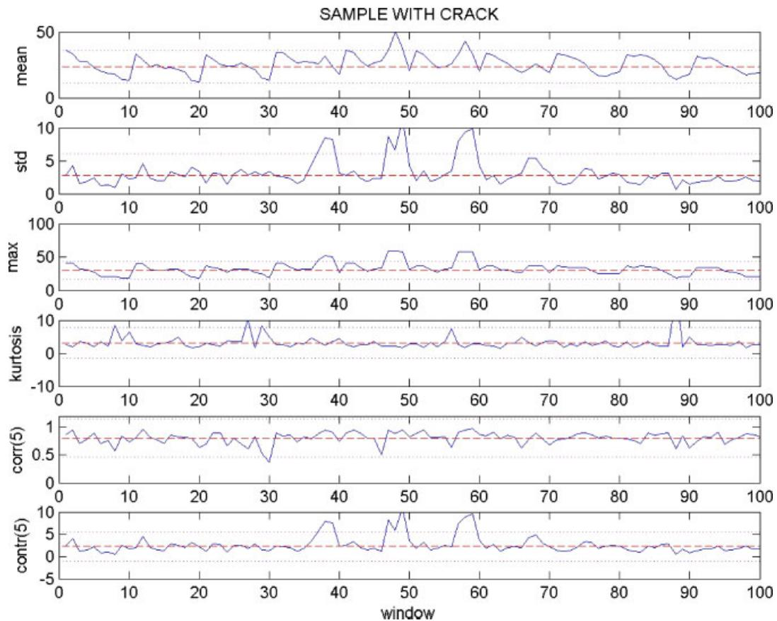
Figure 4. Values of textural characteristics in 100 windows computed from the image of region with a defect (In Li *et al.* Figure 5 above right).
