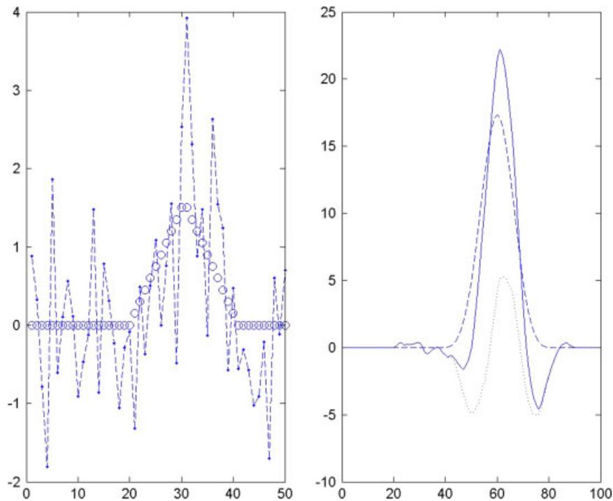
Figure 1. Left: signal (circles) and signal with noise (dots). Right: filtered signal (dashed), noise (dotted), and signal with noise (full).
