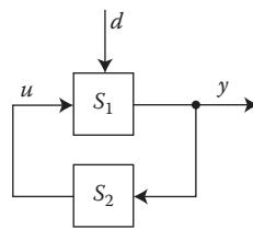
**FIGURE 21.2** Disturbance attenuation.
