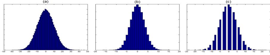
Figure 1. Shown are: (a) the histogram of a non-quantized random values drawn from a zero-mean normal distribution; (b) histogram of the quantized (a) with quantization step  $Q^\alpha = 3$ ; (c) histogram of the double-quantized (a) with quantization steps  $Q^\alpha = 3$  and  $Q^\beta = 2$ .
