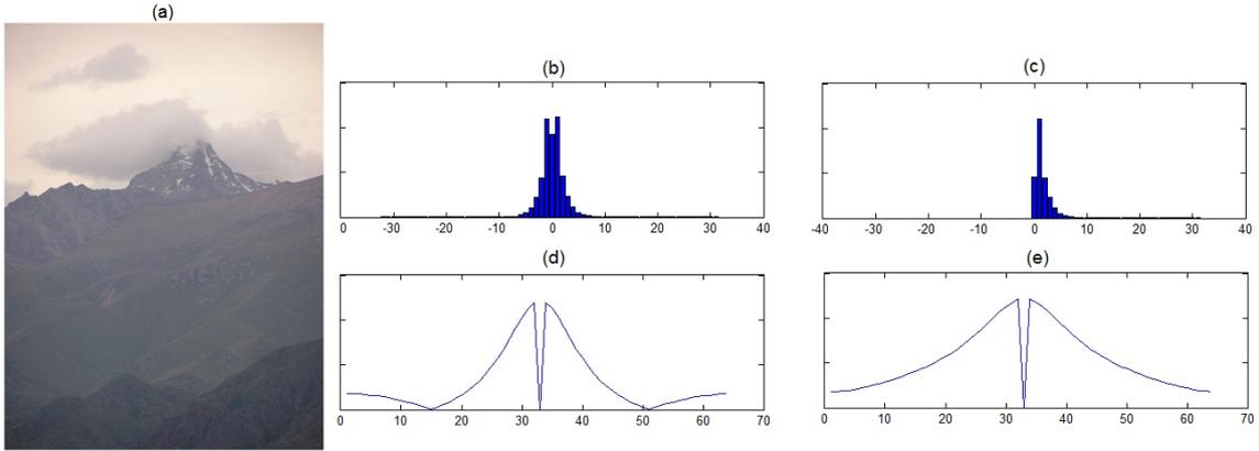
Figure 3. Shown are: (a) the tested single compressed images; (b),(d) outputs of the method described in [10] resulting in a false positive (the spectrum has not the typical decaying trend); (c),(e) output of the method described in this paper. In both cases the method was applied to DCT coefficients corresponding to frequency (1, 0).
