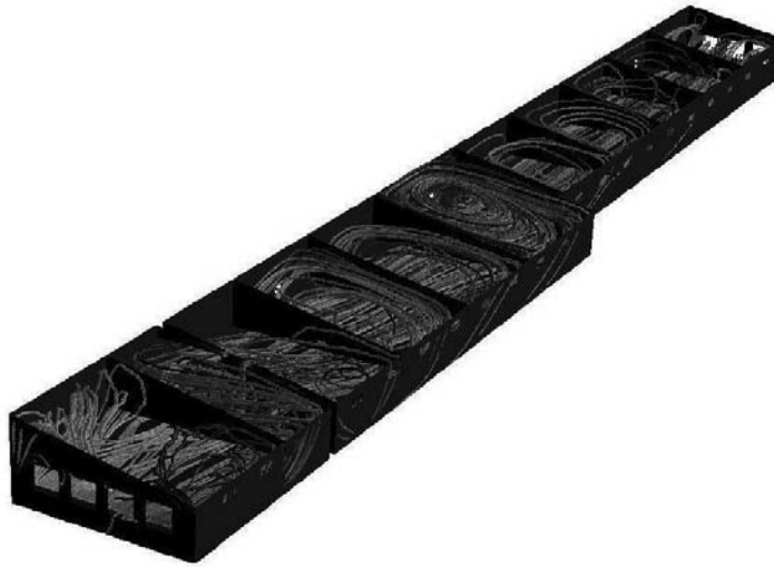
Fig. 4. Pathlines of air obtained during the simulation of longitudinal ventilation.
