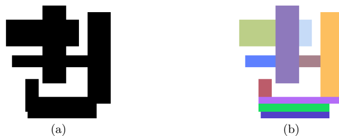
Fig. 5. (a) The binary convolution kernel used in the experiment. (b) Its 10 blocks of GBD decomposition.
