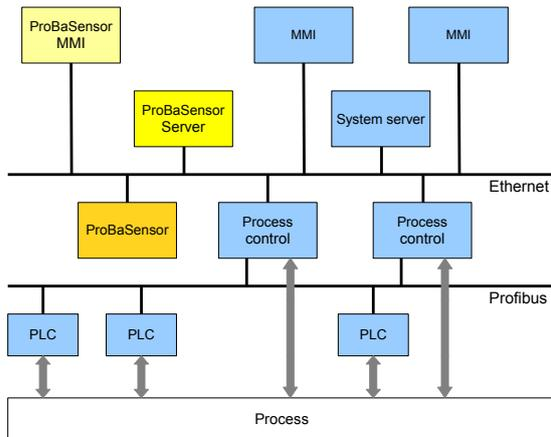
Fig. 2. Scheme of the experimental integration of new nodes into a real control system of a rolling mill.
