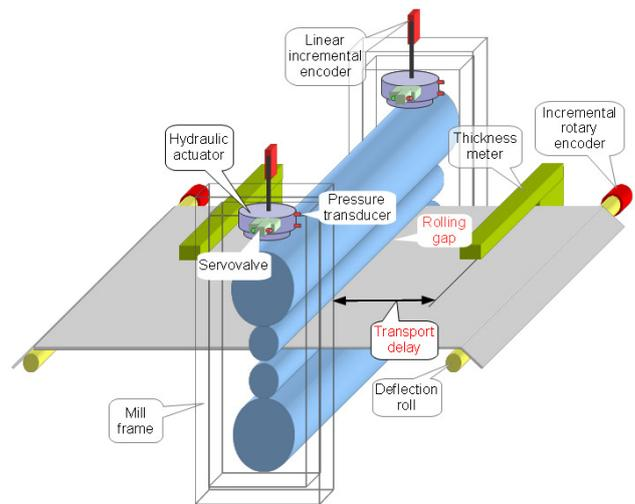
Fig. 1. Scheme of a four-high rolling mill.
