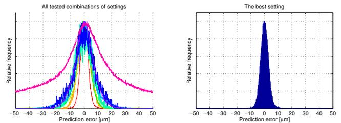
Fig. 8. Histograms of prediction error for experiments on the rolling mill  $S$ .
