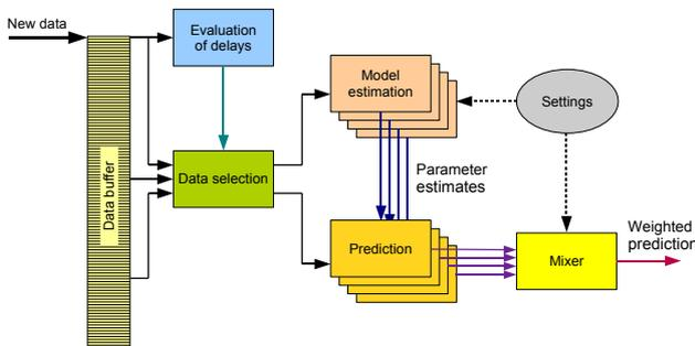
Fig. 3. Block diagram of the ProBaSensor core.
