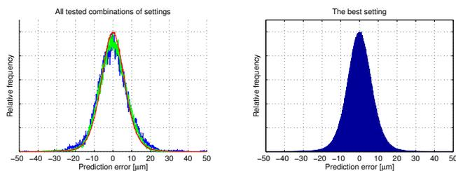
Fig. 9. Histograms of prediction error for experiments on the rolling mill C.
