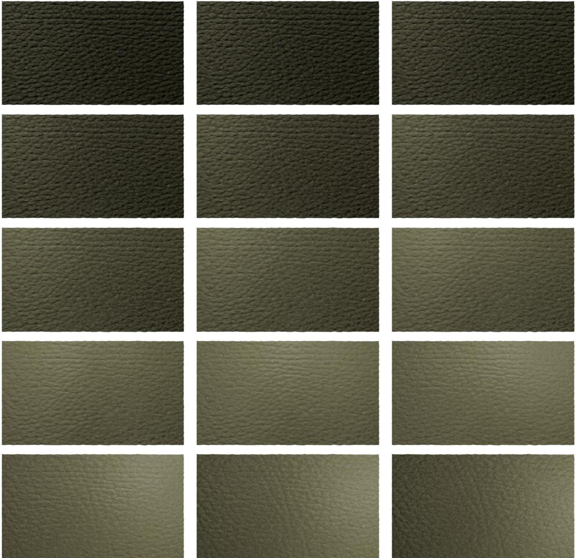
Figure 1: Resulting BTF texture of foil, synthesised texture combined with its range map mapped on bumpy board rendered with 15 different angles of illumination and fixed view angle.
