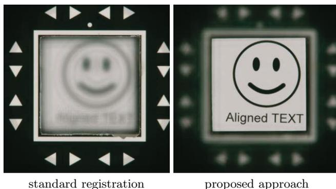
**Fig. 5.** An extreme example of registration based on the reference plane (left) and based on the plane which represents the true surface of the sample found using the proposed method (right) when the heights of the reference plane and the plane of the surface differ considerably. Mean images of the 80 registered images are depicted here.
