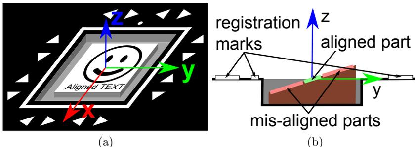
**Fig. 1.** (a) A measured sample, the reference plane with the registration marks (white frame and triangles) and the world coordinate system. (b) a cross-section of (a), shows aligned and misaligned parts of the surface of the measured material when the positions of the reference plane and of the measured surface differ.
