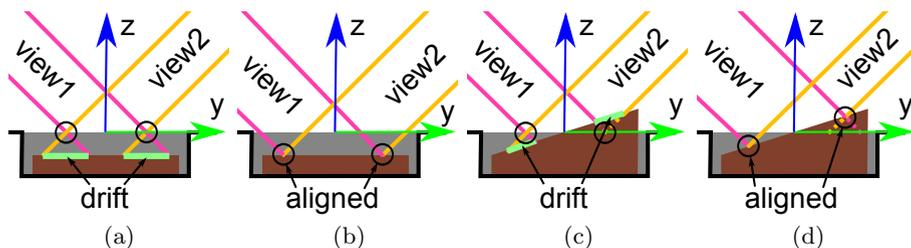
**Fig. 3.** When the plane defined by the registration marks is chosen for registration (a,c), the same pixel will correspond to different points on the surface of the measured sample, i.e., resulting in a small drift. When the appropriate plane on the surface of the material is chosen, the drift disappears (b,d).
