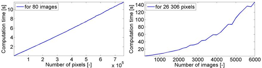
**Fig. 6.** Computational time of one iteration of the algorithm depends on the number of pixels used for quality evaluation (left), and on the number of processed images (right)
