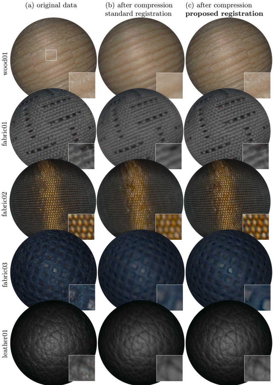
**Fig. 7.** A comparison of BTF visualization: (a) rendering using all 6561 images, (b) and (c) rendering from a compressed representation using only 50 eigen-images without and with application of the proposed alignment method
