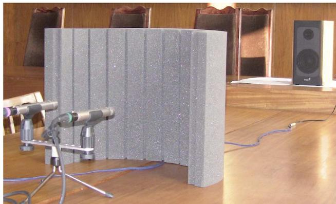
Fig. 5. Photo of the recording situation with the foam obstacle placed 40 cm in front of the microphones. The loudspeaker is located in position 2.
