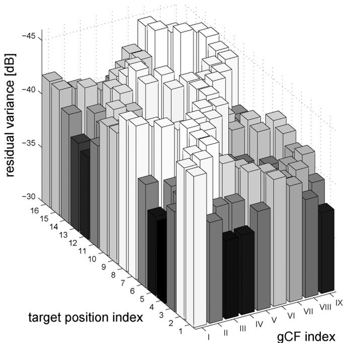
Fig. 3. Residual variances of gCFs' outputs when the female target speaker utters from positions 1, . . . , 16. For example, it is seen that the gCF I yields the best cancellation performance for positions 1, 2, 7, and 8, which corresponds to the filter definition in Fig. 1.
