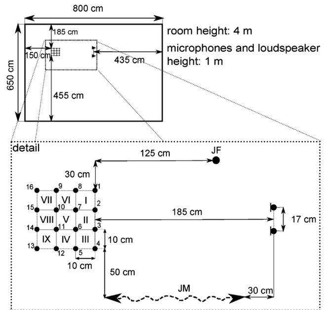
Fig. 1. Setup of the room which was utilized in our experiments. The known positions of the target source, located in a regular grid, are numbered from 1 to 16. The roman numerals correspond to gCFs for the groups of four adjacent positions. For example, the gCF IV is defined for positions 5, 6, 11 and 12.
