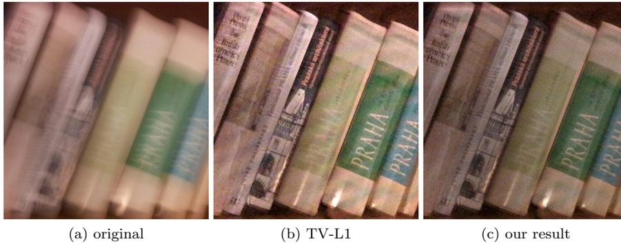
Figure 5: Test 3 — 1/2 s exposure, 72×76 estimated PSF.
