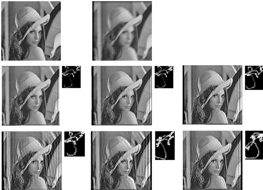
Figure 8: Noise in gyroscope data. Synthetically blurred Lena image using PSF from recorded gyroscope samples and afterwards deblurred using PSF from measurements with variable amount of noise. Images are from left to right, top to bottom: original, blurred and 6 deblurred images using original gyroscope data altered by random gaussian noise with variance from 0 to 0.05 (gyroscope measurements are in rad/s).
