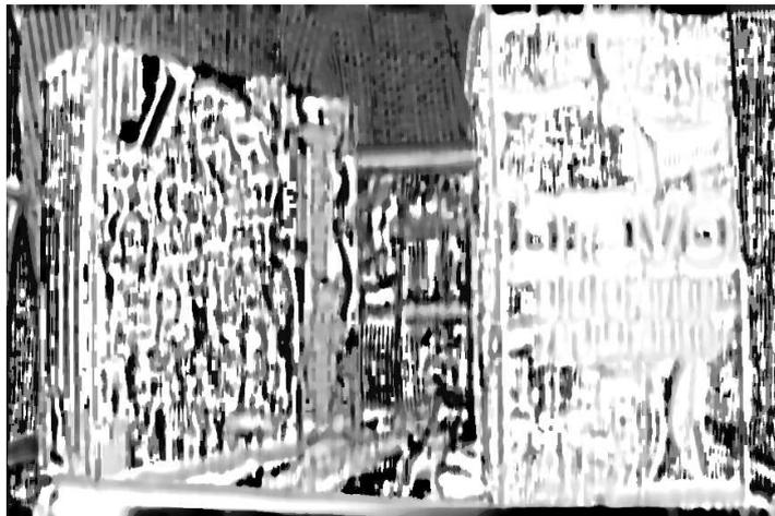
(b) depth map got by Algorithm III, error averaging by  $7 \times 7$  window, result smoothed by  $11 \times 11$  median filter
