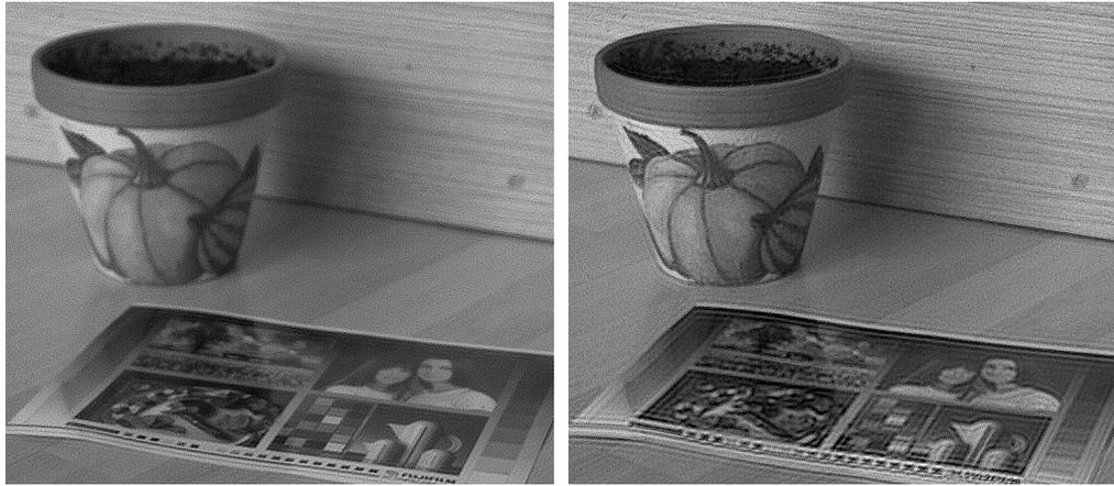
(a) deconvolution using PSFs valid in the lower part of the image      (b) deconvolution using PSFs valid on the wall in the upper-right corner of the image
