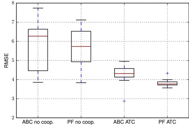
**Fig. 2.** RMSEs of network nodes. The first two boxplots display values for the ABC and particle filter (PF) without cooperation, the third and fourth boxplots display values for the ABC and particle filter with cooperation (adapt-then-combine, ATC).
