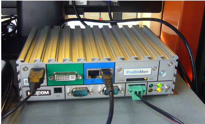
Fig. 7. A node of the ProDisMon condition monitoring system.
