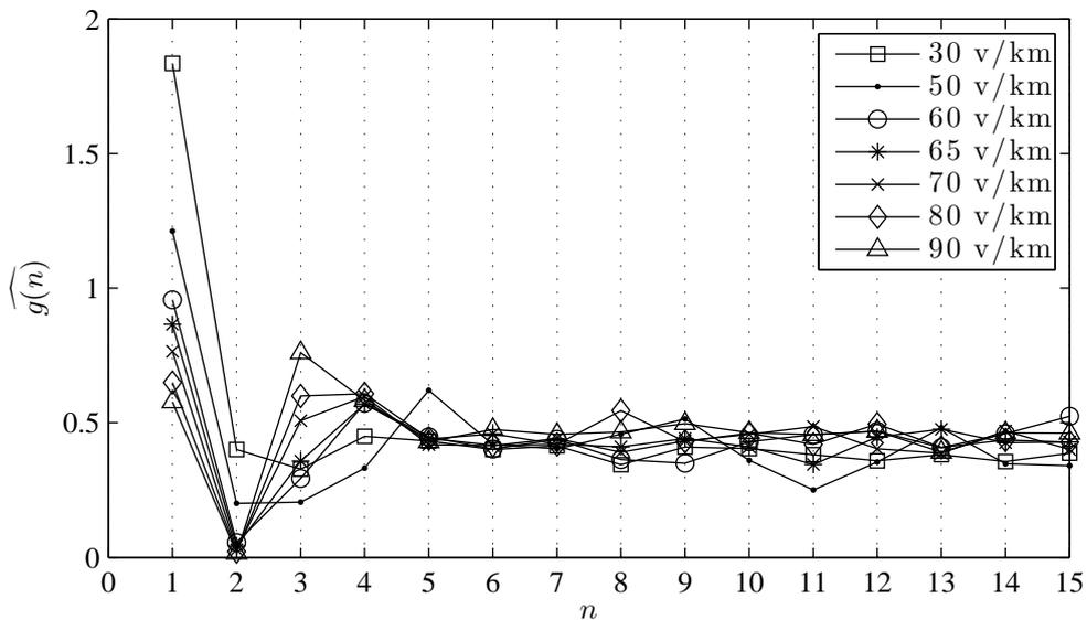
Figure 7: Estimation of hopping rates for various densities.
