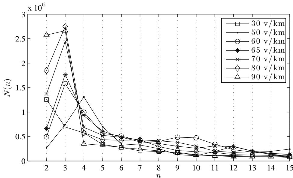
Figure 8: Occurrence of the blocks of the length  $n$  for various densities.
