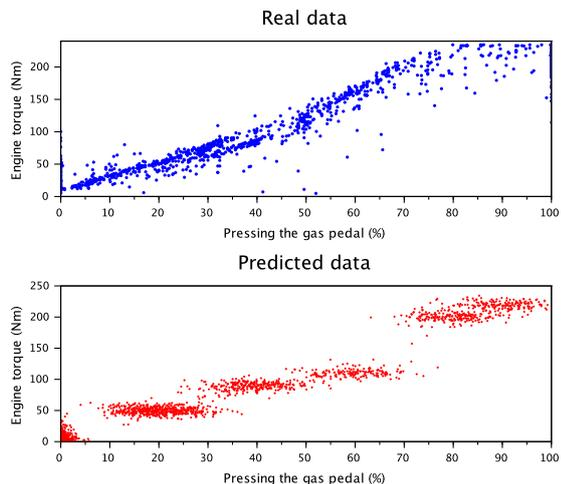
Figure 2. Clusters in the beginning of the estimation. The top figure plots the real measurements of pressing the gas pedal against the engine torque. The bottom figure shows the same for the predicted data. Notice 6 visible clusters in the bottom figure.
