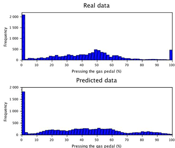
Figure 4. Histogram of real and predicted data. Notice frequencies of the clearly visible one exponential component near zero values. The rest of them correspond to five normal components. Notice correspondence of the predicted data in the bottom figure to the original real data in the top figure.
