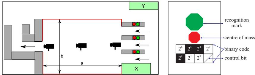
**Fig. 1.** Taken from [6]. Left: Experimental setting the experiment,  $a = 7.2$  m,  $b = 4.4$  m. After the passage through the exit, participant returned to the area Y waiting for another entry. Right: sketch of pedestrian’s hat used for automatic image recognition.
