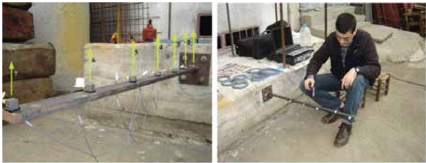
Figure 7. Cantilever beam model, acceleration set-up, and excitation with a hammer.
