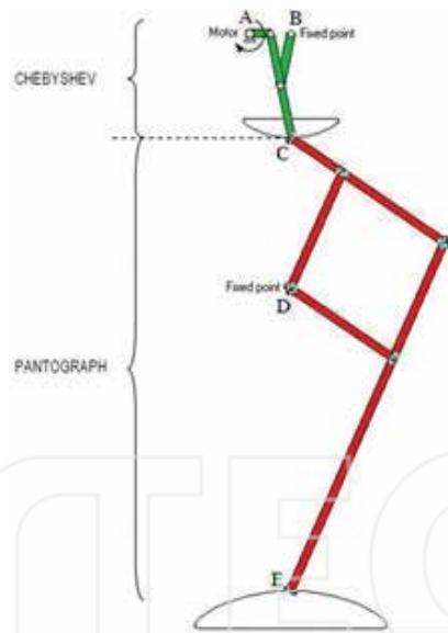
Figure 3. The sub-mechanisms Chebyshev and pantograph with the trajectories of their notable points.
