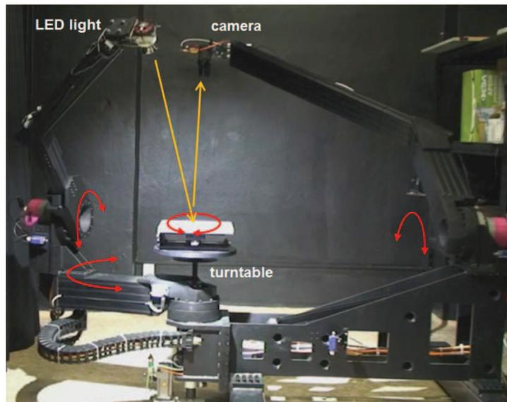
**Figure 2 – UTIA gonioreflectometer for reference BTF measurements**
