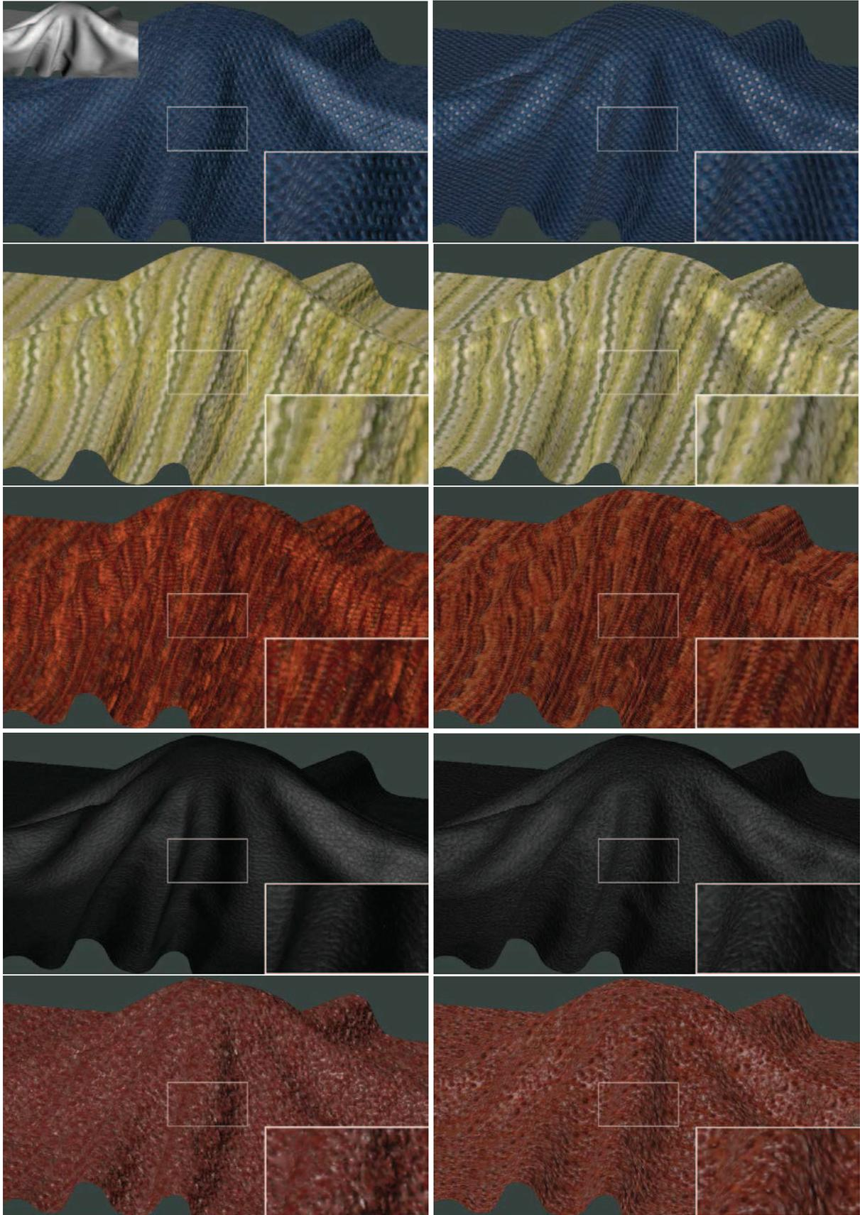
**Figure 7 – A comparison of BTF captured by the reference goniometer in 20 hours (left), and using the portable device in 5 minutes (right)**
