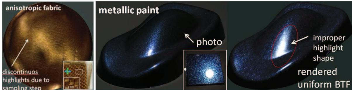
**Figure 8 – Highly anisotropic and specular material measurement challenges**
