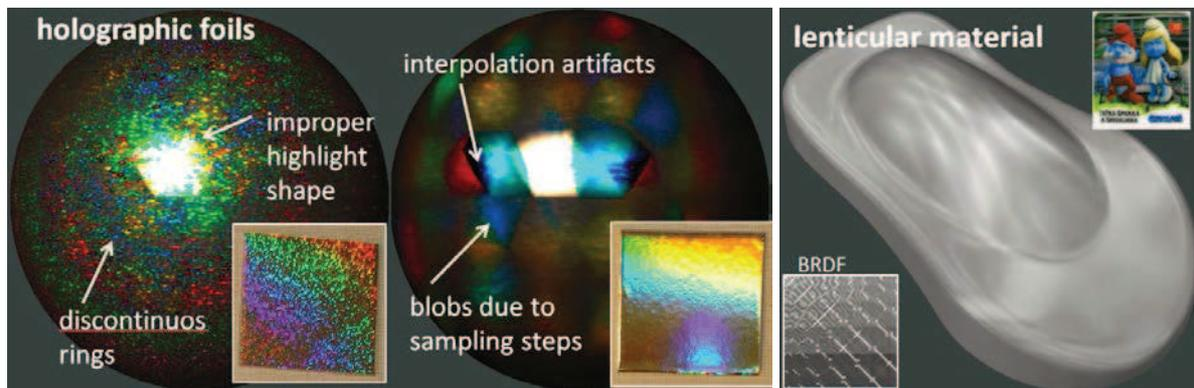
**Figure 9 – Holographic and lenticular materials measurement challenges**
