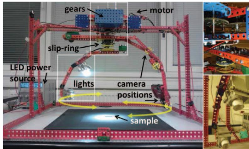
**Figure 4 – Proof-of-concept of fast and portable BTF measurement device**
