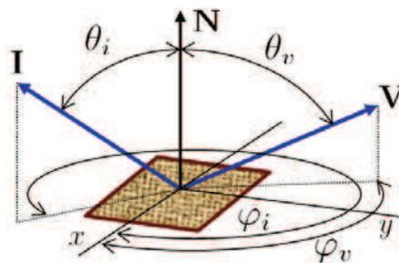
**Figure 1 – A BTF parameterization over material surface**
