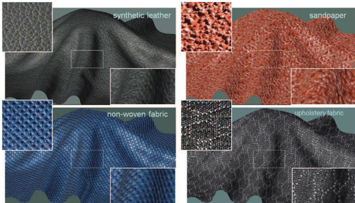
**Figure 5 – Materials captured by the portable BTF measurement device: leather, sandpaper, fabric**
