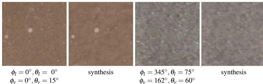
**Fig. 4.** An example of the measured BTF terracotta texture and its synthetic (even images) results, where  $\phi, \theta$  are azimuthal and elevation illumination / viewing angles, respectively.
