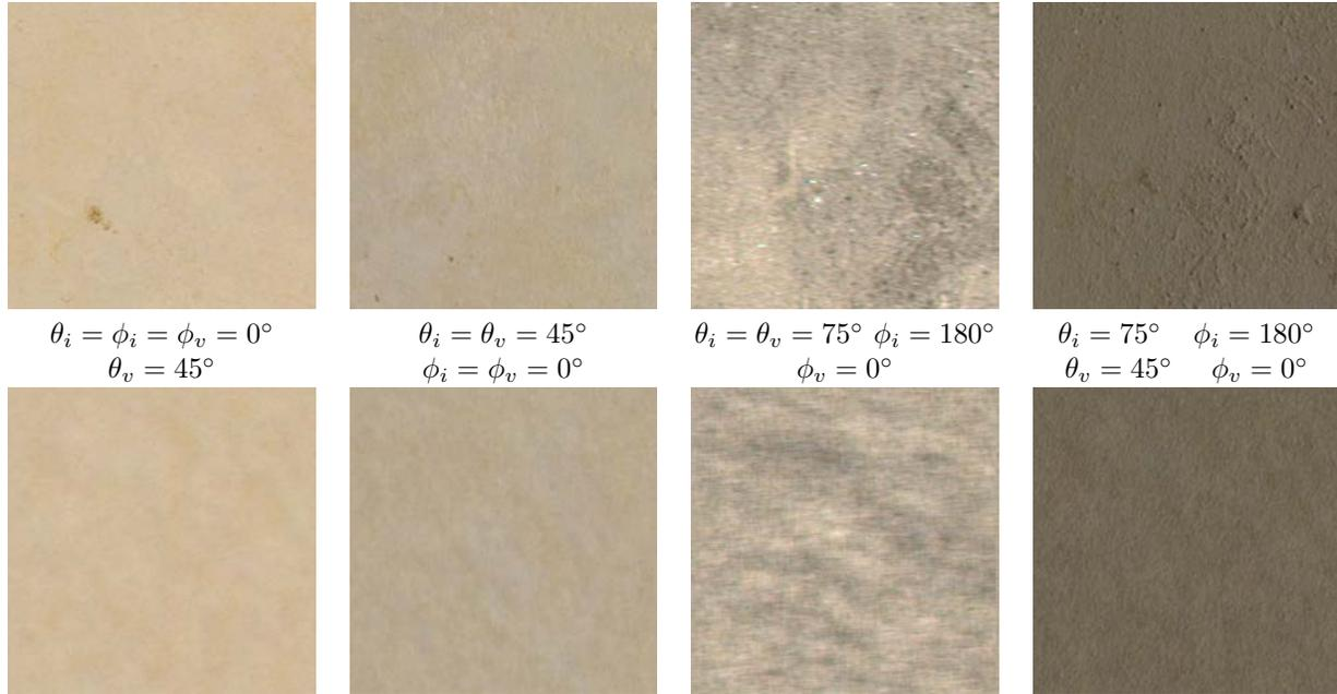
**Fig. 1.** BTF plaener texture measurements (upper row), their synthetic counterparts (bottom row) for various elevation ( $\theta_i, \theta_v$ ) and azimuthal ( $\phi_i, \phi_v$ ) illumination and viewing angles.
