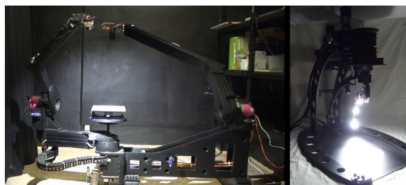
Figure 1: Gonioreflectometers used for capturing of material appearance at UTIA: (left) the reference, (right) its portable counterpart for rapid appearance acquisition.
