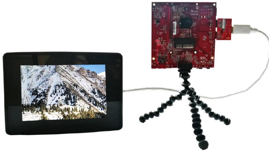
Fig. 2. Complete camera-to-touchscreen demo kit
