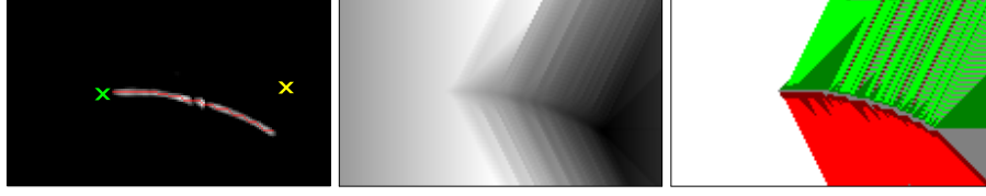
Fig. 2. Example of dynamic programming. Estimated discrete trajectory P is marked in red, starting point \mathcal{C}_{t_{s-1}}(0) by green cross, and ending point \mathcal{C}_{t_s}(1) by yellow cross. These points were deliberately moved further away to show robustness of the approach. Left image: accumulated blur kernels from two consecutive frames H_{t_{s-1}} and H_{t_s} in joint coordinate system. Middle image: value of the energy function at each pixel from black (lowest) to white (highest). Right image: pixels where moving down by 1 is optimal are marked in dark green, down by 2 in bright green, up by 1 in dark red, up by 2 in bright red and moving straight in grey. Pixels, where reporting a starting point x_b is optimal, are white. The minimal value of the energy function is at the most right red pixel x_e in the left image. The whole trajectory is then estimated from right to left by backtracking until the next minimizing pixel is reported as a starting point (white space).
