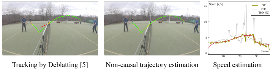
Fig. 1. Trajectory reconstruction using the proposed non-causal Tracking by Deblatting (middle) compared to the causal TbD [5] (left). Color denotes the trajectory accuracy, from red (complete failure) to green (high accuracy). Ground truth trajectory (yellow) from high-speed camera is shown under the estimated trajectory. Speed estimation is shown on the right. Ground truth speeds (olive) are noisy due to discretization and TbD speed estimation (lightgray) is inaccurate, which is fixed by the proposed TbD-NC (purple).
