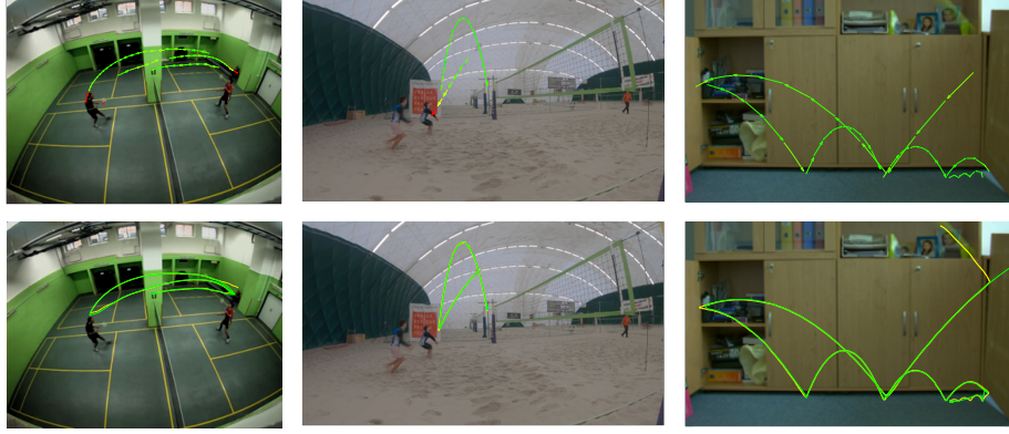
Fig. 4. Trajectory recovery for selected sequences from the TbD dataset. Top row: trajectories estimated by the causal TbD [5] overlaid on the first frame. TIoU (7) with ground truth trajectories from a high-speed camera is color coded by scale in Fig. 3. Bottom row: trajectory estimates by the proposed TbD-NC which outputs continuous trajectory for the whole sequence. The yellow curves underneath denote ground truth. Arrows indicate the direction of motion.
