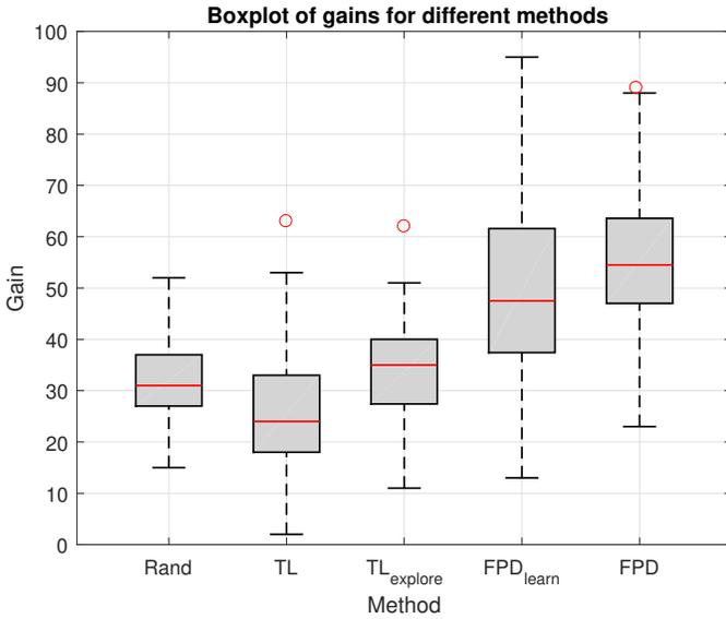
Fig. 1. Boxplot of gains, data gathered with ideal model  $I\tilde{p}_3$ . Rand - random policy, TL - TL method,  $TL_{\text{explore}}$  - TL method with exploration,  $FPD_{\text{learn}}$  - learning FPD method, FPD - FPD method with complete knowledge.
