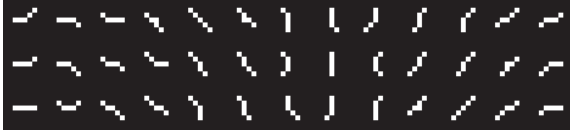
Fig. 2. Proposed atoms: 36 line segments of length 5 used to build the atomic set A .
