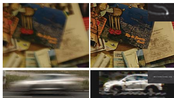
Fig. 1. Real examples of motion blur caused by camera motion (top) and by object motion (bottom). Blurred images (left) and estimated sharp images (right) with zoomed blur kernels shown in insets.
