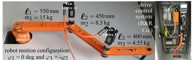
Fig. 9. Realized laboratory model of robot arm in scale 1:4.
