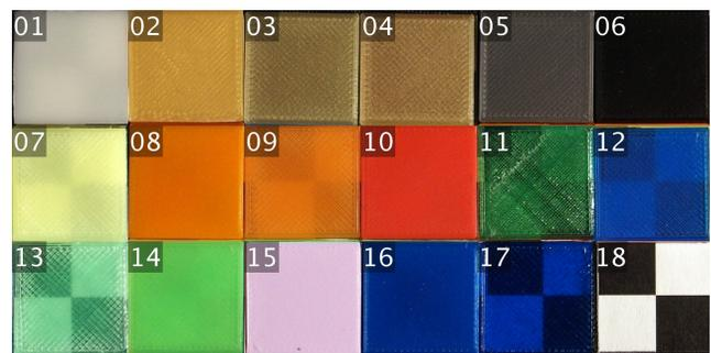
Fig. 2. 3D printed tiles of height 1mm used in the psychophysical study.
