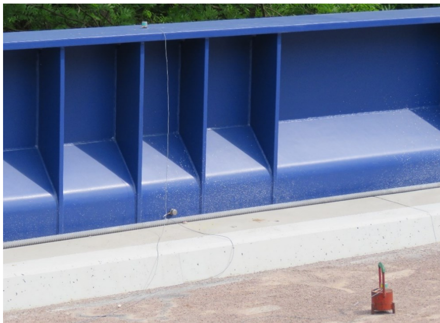
Figure 4. The view on the three accelerometers of type 8344 placed on the main girder and on the roadway.
