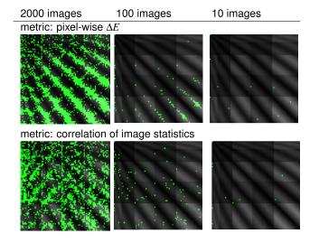
**Figure 10.** Maps of the preserved BTF images for two tested metrics and their three different thresholds preserving 2000, 100, and 10 images. The preserved images are shown as green dots in BTF space of 81 illumination (rows) and 81 viewing (columns) directions.
