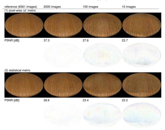
Figure 11. A comparison of BTF renderings for all images with their reduced variants for three reduction thresholds (columns) and two different reduction metrics (rows). Attached are the difference images from the reference.
