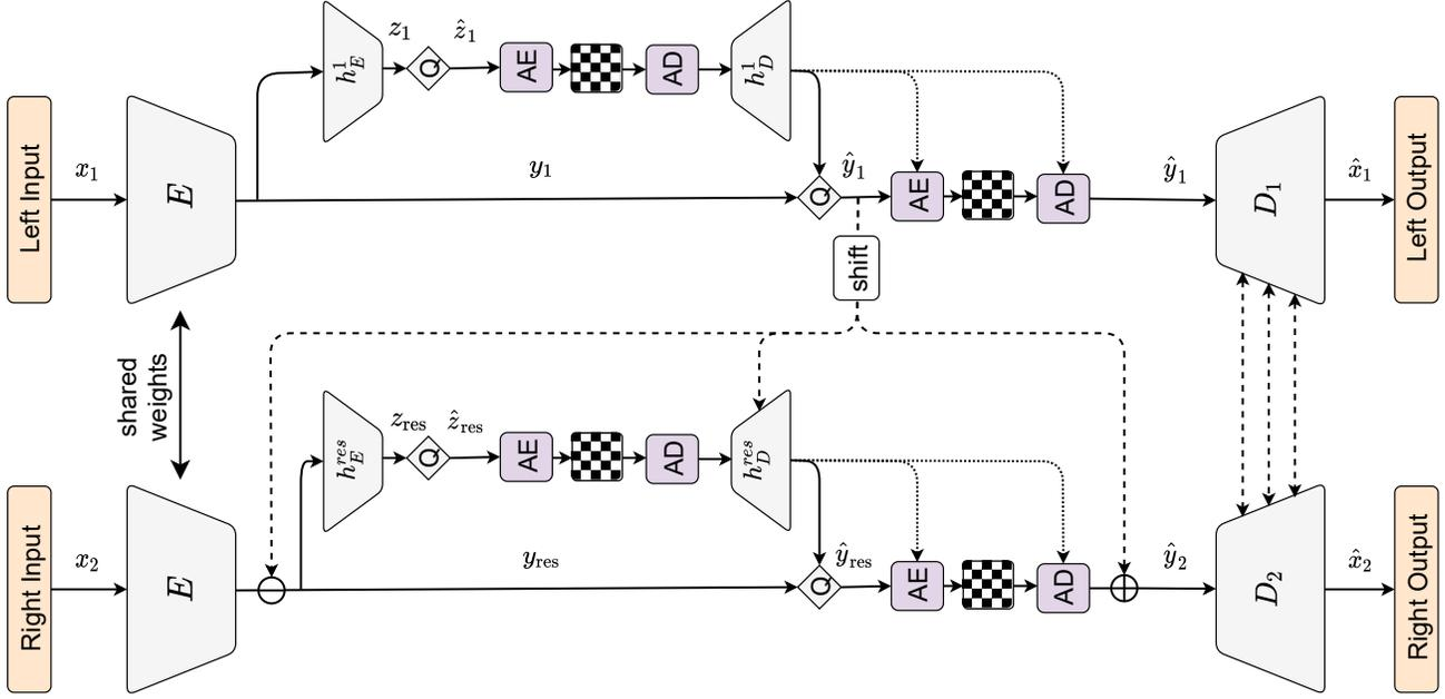
Figure 1. The full architecture of our proposed method. Layer structure of submodules are shown in Fig. 2 and Fig. 3. The arithmetic encoder AE and the arithmetic decoder AD are not relevant during training. The bitstreams are pictured with a checkerboard pattern. Dotted lines are connections not relevant during training and dashed lines show connections between the left and the right side.
