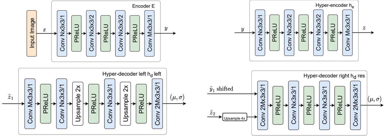
Figure 2. The top row shows the architecture of encoder  $E$  and hyper-encoder  $h_E$ . The bottom row shows the decoder of the hyperprior with the decoder for the left image bottom left and the decoder for the right image bottom right. We set  $N = 192$  and  $M = 12$
