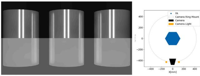
**Fig. 4.** The difference between local (top) and global (bottom) illumination is depicted. The dark background represents the surface of an inspection chamber, appearing nearly black with local illumination and gray with global illumination. The image highlights the significant impact that proper lighting has on the material's appearance. The local illumination setup resembles the configuration of real-world camera mounts (right) used during inspections.
