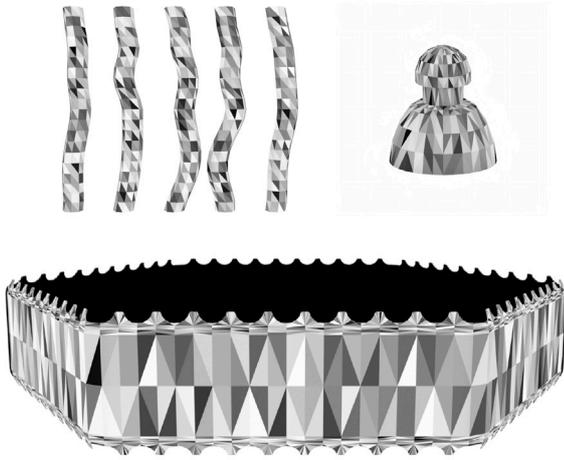
Fig. 2. The mesh of the fuel rods (left) is composed of segments that are displaced in the  $XY$  plane based on the generated rod divergence curves. The right image displays the mesh of a fuel rod tip. The bottom image shows the mesh of a spacer grid. Note that in all the mesh images, each face is assigned a random color to highlight the 3D structure.
