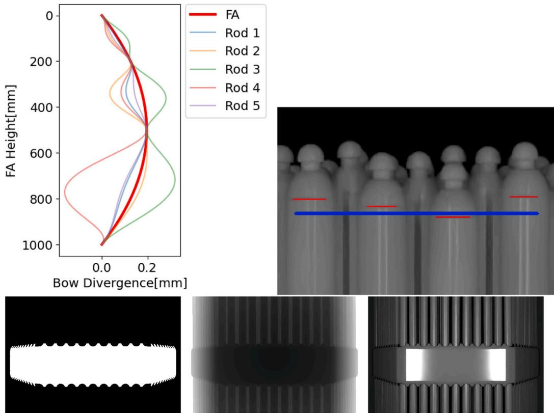
Fig. 6. Ground truth for various aspects of the FA includes: (a) Fuel bow and rod divergence curves; (b) Growth of individual rods (only five are shown); (c) Spacer grid mask (used for semantic segmentation) derived from frame (d); (d) Depth map corresponding to the same spacer grid.
