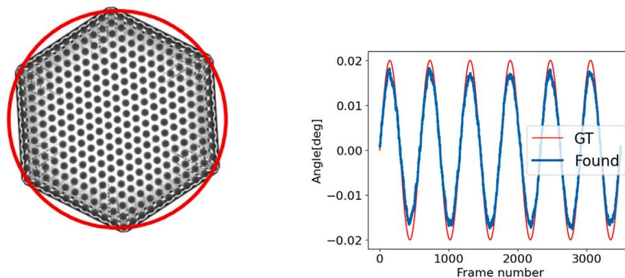
Fig. 8. The figure shows circle around FA's top (left) and swinging angle compared to ground-truth (right). The close match between the two demonstrates the accuracy of the synthetic dataset in replicating real-world fuel assembly movements.
