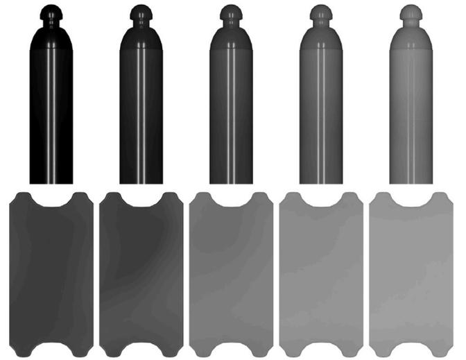
Fig. 3. Fuel rod cladding made of zirconium alloy (top) and spacer grid material made of Inconel (bottom) are shown with varying parameters to illustrate surface changes in aging fuel, ranging from the newest (left) to the oldest (right).
