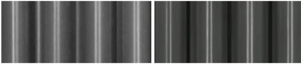
Fig. 1. Comparison of frames from real (left) and synthetic (right) nuclear fuel inspection videos. The synthetic sample does not contain any camera distortion therefore the image can be post-processed to further resemble the real-world images.
