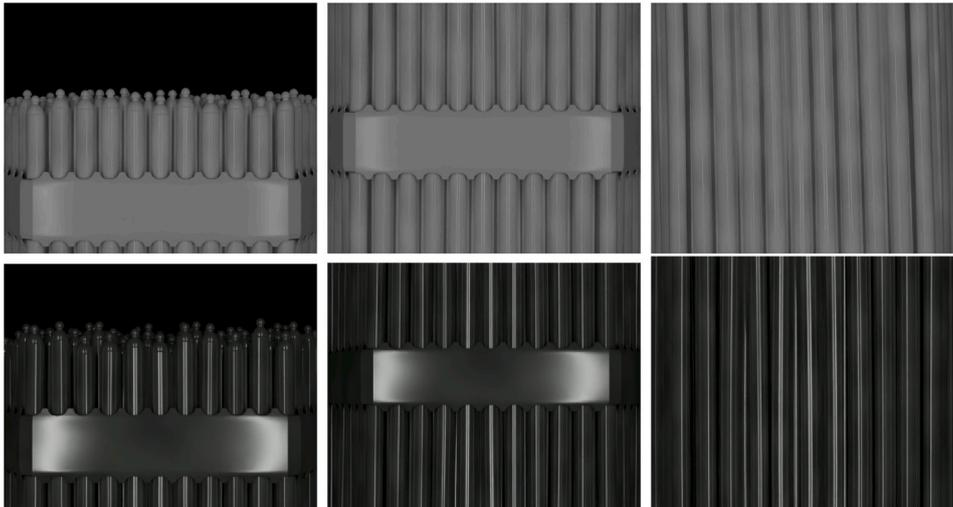
Fig. 5. Example frames from fuel with high (top) and low (bottom) levels of oxidation.
