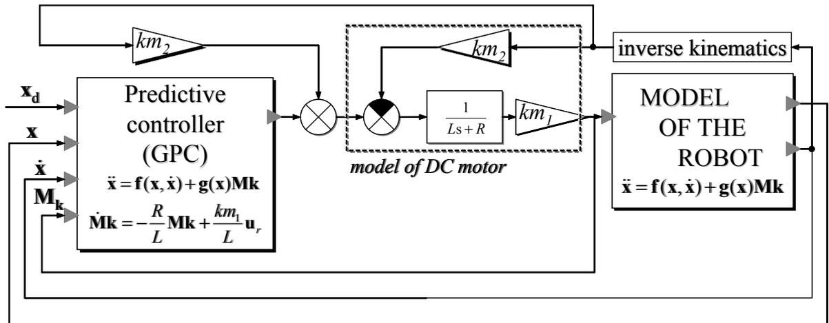
Fig. 4. Scheme of control circuit with predictive controller applied to global model.
