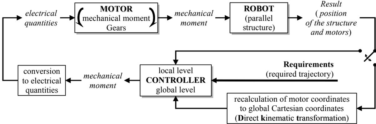
Figure 2. Conceptual scheme of control circuit for local (independent) and global (centralized) model-based level.
