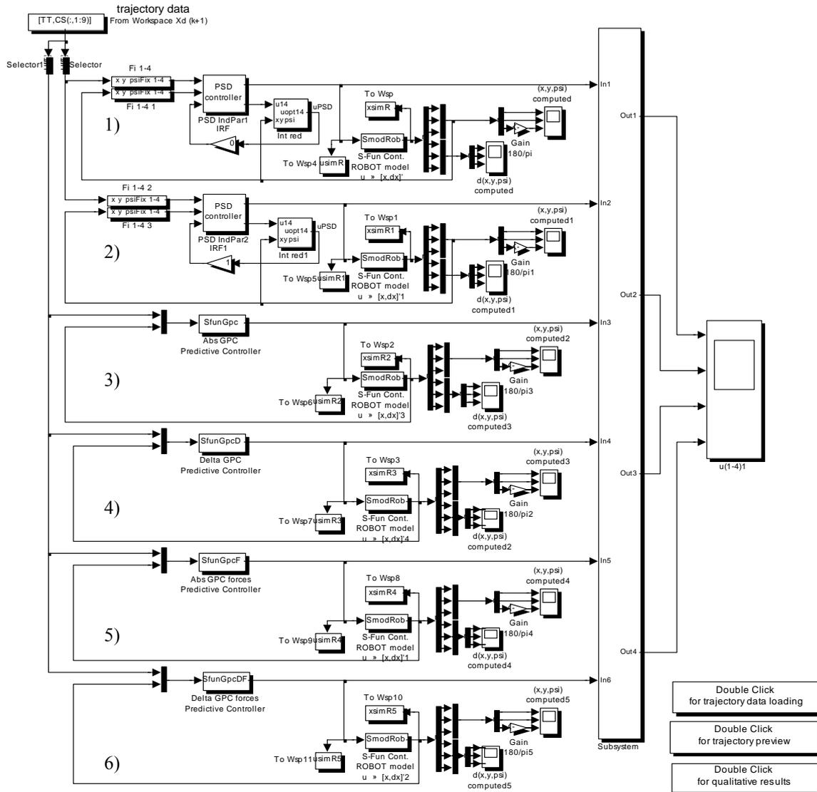
Figure 5. SIMULINK scheme for parallel comparative simulation of PID/PSD controllers and predictive controllers;
