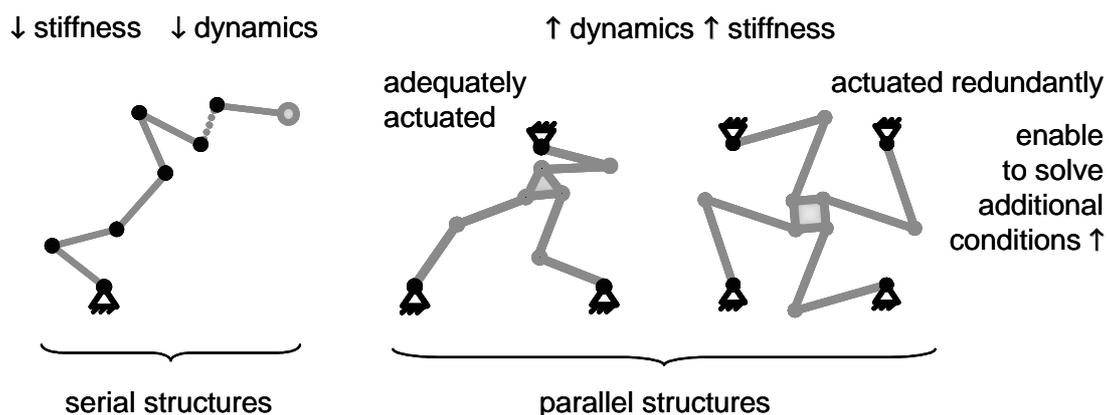
Figure 1. Comparison of serial and parallel structures.
