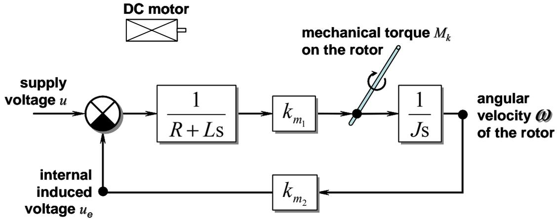
Figure 3. Block scheme of brushes DC motor with permanent magnet in the stator.
