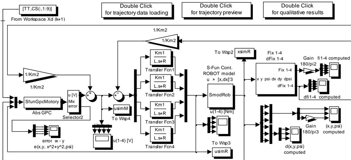
Figure 6. Control circuit with global robot model.
