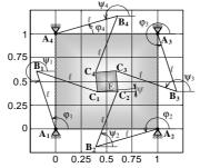
It consists of the basic frame, which at the same time encloses workspace of the robot, four independent drives, movable platform and eight arms, which connect the movable platform with the basic frame. The arms are parallely situated.
