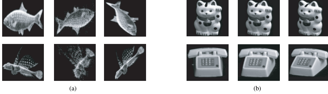
Figure 1. (a) Samples of fish images. From left to right: original images, affine and Gaussian noise distorted images (std 10 % of maximum intensity), and affine distorted and occluded images (occlusion size 5 % of image side). (b) Samples of Coil-100 images at angle 0, 10, and 20 degrees.
