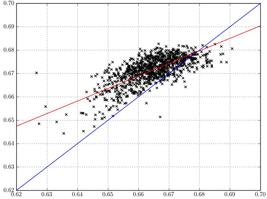
Figure 3: Scatterplot  $H_2/H_1 \times v_r$  with line of theoretical dependence (blue) and real linear regression line (red).
