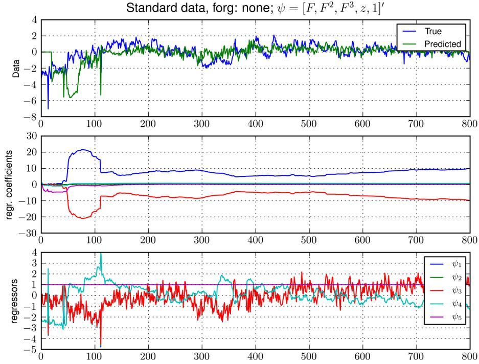
Figure 7: Gaugemeter model – 3rd order – normalized data
