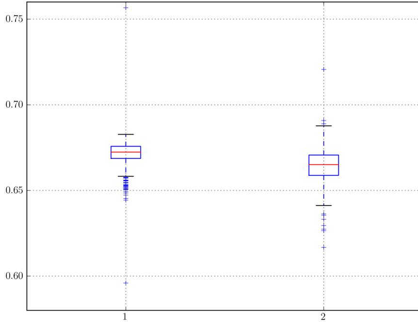
Figure 2: Boxplots of  $H_2/H_1$  (1) and  $v_r = v_1/v_2$  (2), respectively. The blue box extends from the lower to the upper quartile, hence it contains 50% of data samples. The red line is the median. The whiskers show the range of the data, their length is 1.5IQR (inter-quartile range). + denote outlier data w.r.t. quartiles.
