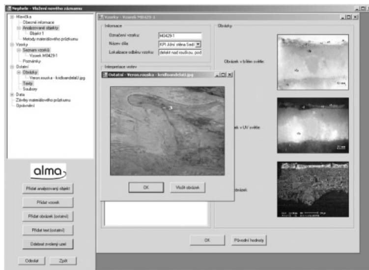
Figure 9. An example of the proposed system GUI. The overview image of the painting together with the three modality images – VIS, UV, and SEM data – are presented here.
