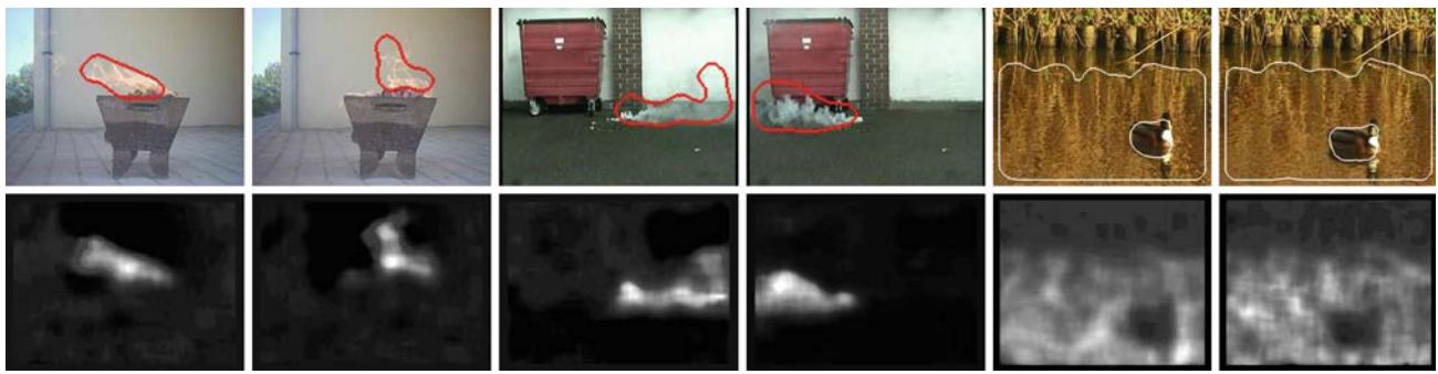
Fig. 1 Top row: Sample frames of three video sequences with the dynamic texture regions detected. The videos were acquired by static camera. Bottom row: The optical flow residual maps
