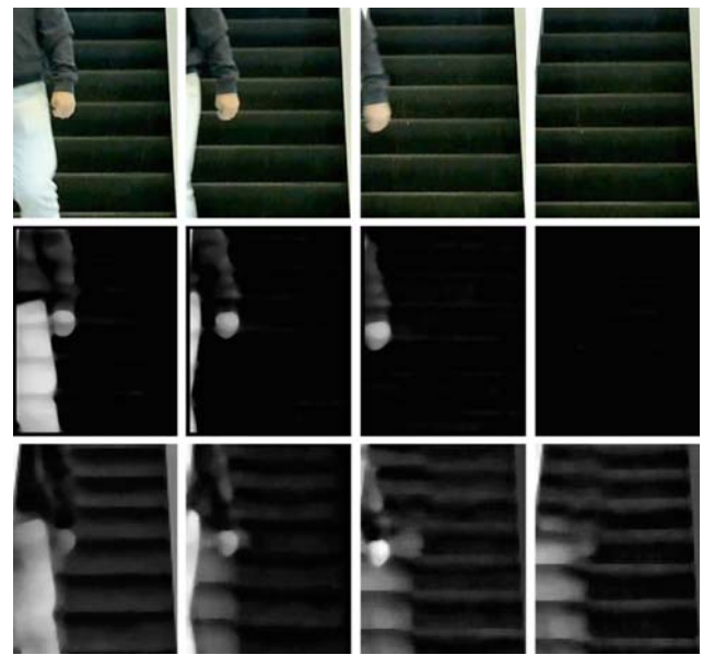
Fig. 10 Top row: Sample frames of the ‘Man and Escalator’ sequence. Middle row: The resonant residual maps. Bottom row: Residual maps obtained in a sliding temporal data window with unit temporal spacing
