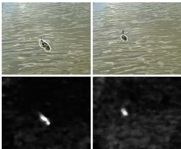
Fig. 5 Sample frames of the ‘Duck’ sequence. Top row : Results of target detection using our method with photometric invariants. Bottom row : Residual maps
