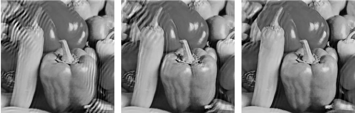
Figure 1.7: Deblurring of the right image from Fig. 1.4 using (from left to right) 1, 2 and 3 kernels per image width. Obviously the occurrence of artifacts decreases with the number of kernels.
