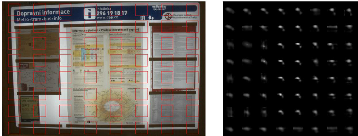
Figure 1.12: First of six input images ( $1700 \times 1130$  pixels) used for super-resolution (left) and  $8 \times 8$  local convolution kernels computed by the SR algorithm [39] (right). Spatial variance of the PSF is obvious. Squares in the image depict patches, in which the kernels were estimated.
