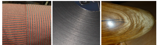
Figure 2: Real-world examples of anisotropic appearance of materials: fabric, machined plastic, and polished wood. Anisotropy is caused by the orientation of different threads of fibers, parallel grooves (causing highlight perpendicular to their direction), and wooden fibers (exhibiting both specular (left) and anisotropic (right) highlights), respectively.
