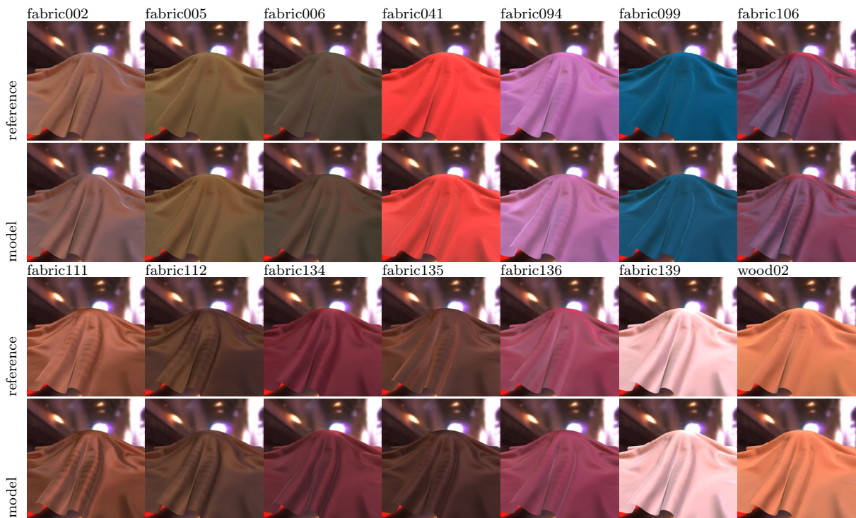
Fig. 11 Comparison between reference BRDF (odd rows) and proposed BRDF model (even rows) renderings in grace illumination environment for 14 tested BRDFs
