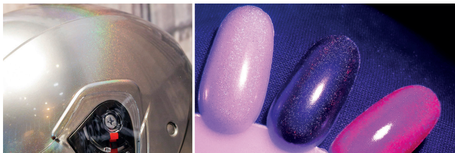
Figure 2. Left: Photograph of a motor-bike helmet: Realisation of chrome-like effects without using chromium 9 by using vacuum metallized pigments (VMPs, Decomet) plus MultiFlect effect pigments in the paint formulation. Right: Alegrace Spectacular effect pigments in nail lacquers (© pictures by Schlenk Metallic Pigments GmbH)
