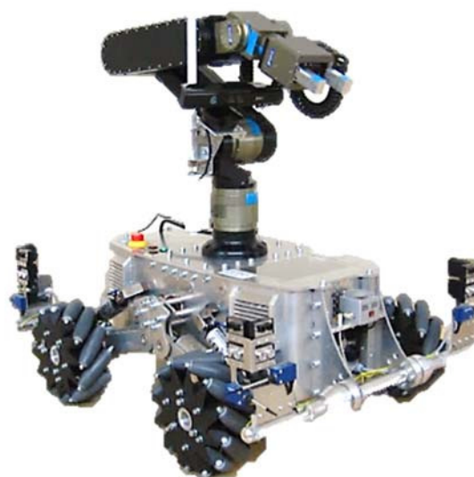
Fig. 1. Overall view of the mobile robotic system: 3 DOF mobile underframe with 5 DOF robot arm [5].
