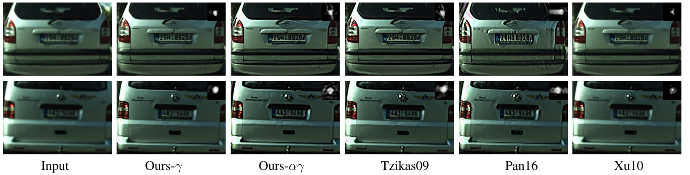
Fig. 13. Real out-of-focus blur, each row represents a new experiment (different photo with different blur). Estimated PSFs superimposed in the top-right corner. Best viewed on computer screen.
