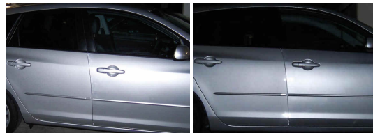
Figure 1: Example of a car body part visually different from the rest of body due to an insufficient number of illumination/viewing validation angles.
