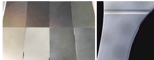
Figure 6: An example of cloudiness / mottling visible as spatial nonuniformity on: (left) a set of coated panels, (right) a part of a car body.
