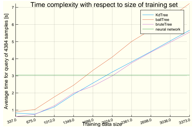
Figure 5: Anomaly detectors’ prediction time dependence on training data size in application phase. Tested on magic telescope and Isolet data sets. Neural model prediction speed does not depend on training data size (note the close-to-zero time in magic telescope case)
