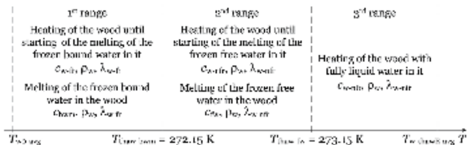
Figure 1. Temperature ranges of the logs' thawing process at u > u_{fsp} and thermophysical characteristics of the wood and of the frozen and nonfrozen bound and free water in it.
